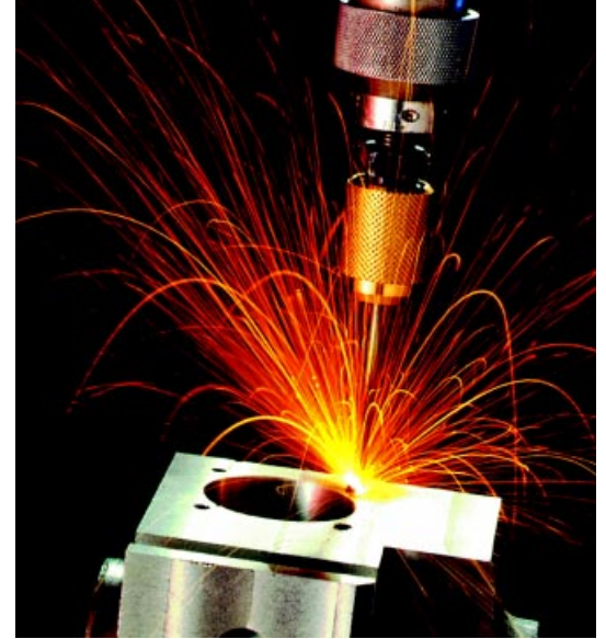
An Electro Arc "Q" type disintegrating head in action, shown without the protective shield normally used to contain coolant and debris.
